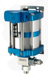
The Autoclave ASL series of pumps are grouped around the 6 inch air piston and then by the actual ratio of air to hydraulic pressure. Inside that group are both single and double air-drive pistons (denoted by the -01 or -02 in model number). A double air piston can increase the liquid output pressure or decrease the required air pressure to get the same amount of "work" from the pump. All Autoclave pumps utilize all-stainless steel wetted parts with an all-aluminium air housing.
